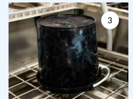
1: Chamber holder for Gallus chambers, 2: Chamber holder for Nilpeter chamber, 3: Rotating nozzles can be placed on the grid for cleaning of buckets.
