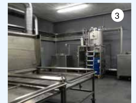
1: Cleaning of hoses 2: Racks for ink trays and doctor blades, 3. Distillation systems and integration between parts washer, tanks, and distiller.
