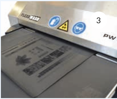
1: Instead of a tray you can add a table for unloading of plates. 2: Sponge roll holder for easy and safe storage of the sponge preventing it from drying out when not used over a longer period of time, 3: With the DLE version you can clean laser engraved plates.
