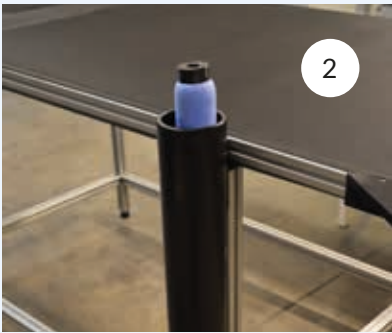
1: Instead of a tray you can add a table for unloading of plates. 2: Sponge roll holder for easy and safe storage of the sponge preventing it from drying out when not used over a longer period of time, 3: With the DLE version you can clean laser engraved plates.
